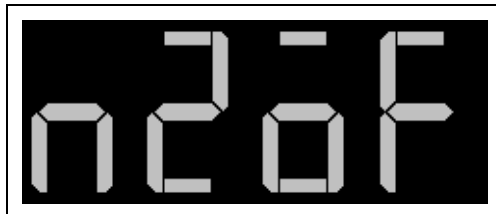
Figure 5. Controller 2 is inactive
