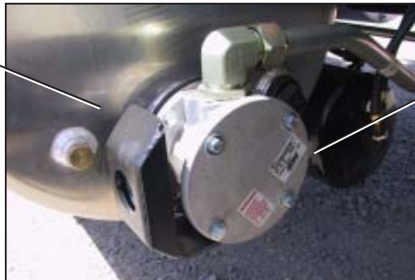
The sample coupler is located at the back of the filter cover.
