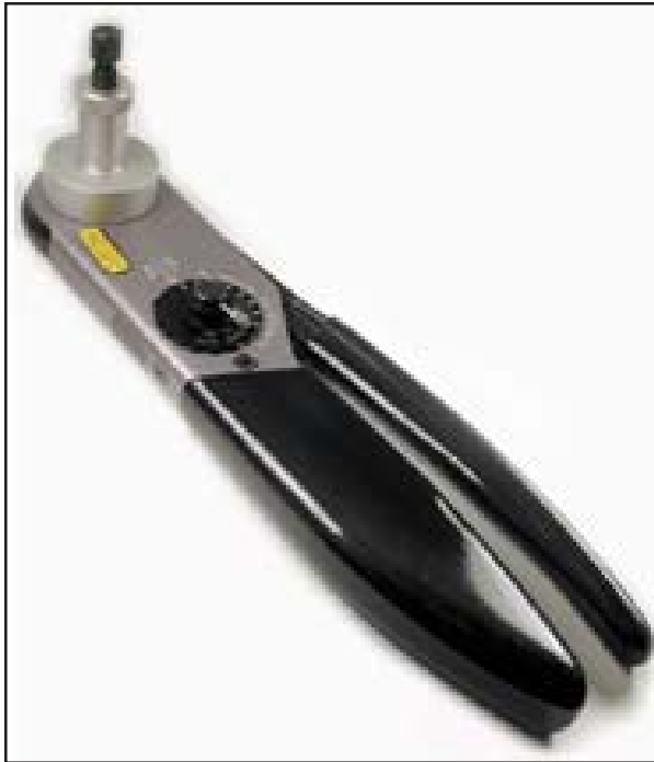
Crimp tool for Deutsch connectors
