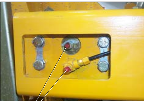
Telescopic arm bearings and rollers
