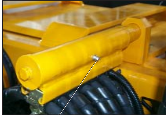
Hoses bracket on the telescopic arm
